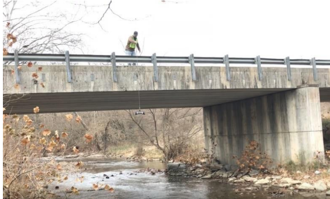
Photo: WVCA staff conduct water monitoring along Indian Creek. At site 5 a Van Dorn horizontal sampling bottle is lowered from the bridge into the stream. Once
