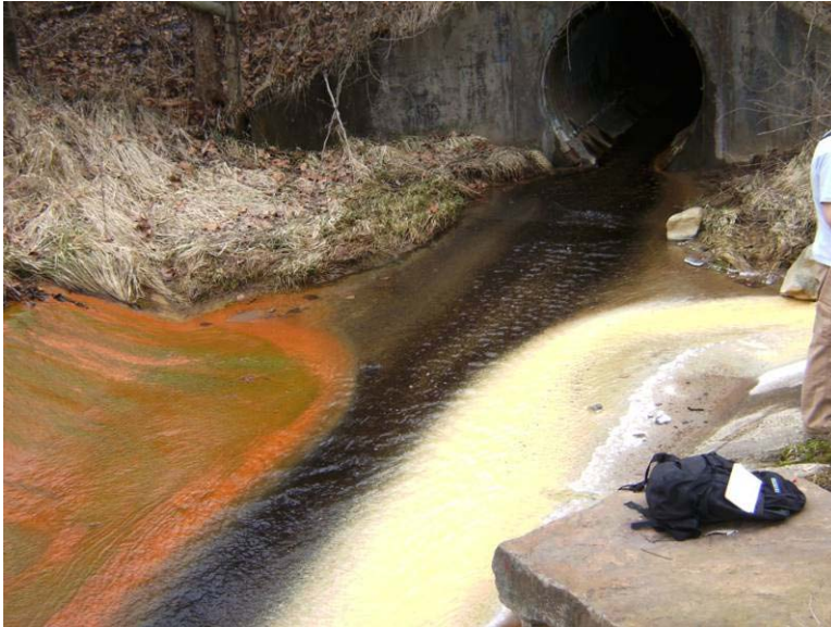
Figure 18: This photograph shows the confluence of three tributaries at “Rainbow Run”. The discharge to the left has high dissolved iron content, while the discharge to the right has high aluminum content. The tributary in the middle has a high pH, low conductivity, and low dissolved metals
