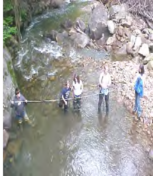
Students prepare to measure a cross-section and discharge during an early fall workshop near the mouth of Wolf Creek.
