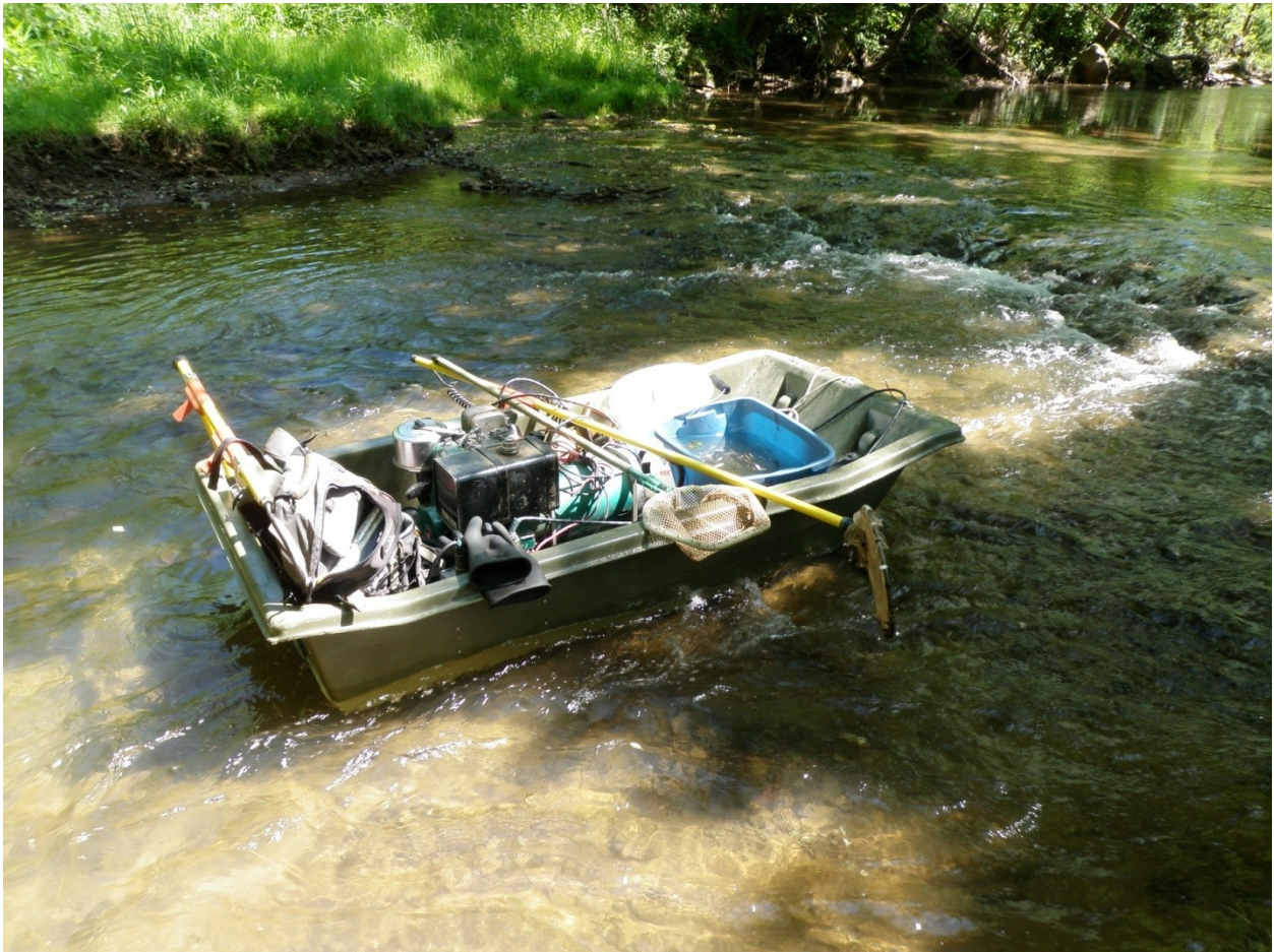
Figure 61. Tow barge with generator, live well, and shocking wand.
