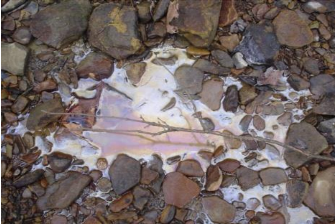
Figure 2-10. Example of Manganese sheen that resembles a true oil sheen in its rainbow coloration.
