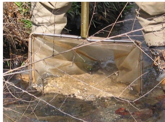
Figure 5-3. Photo of Rectangular Frame Dip Net being placed on stream bottom
