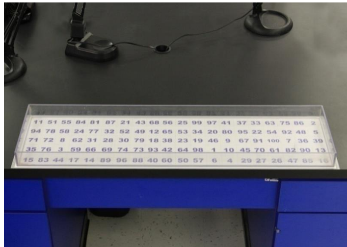
Figure 5-12. Photograph of a Home-Made Gridded Sorting Tray featuring a random number matrix on the bottom.
