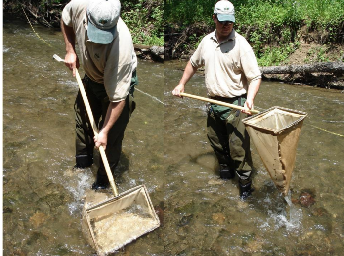
Figure 5-7. Photographs showing the removal of the net from the water with an upstream motion.
