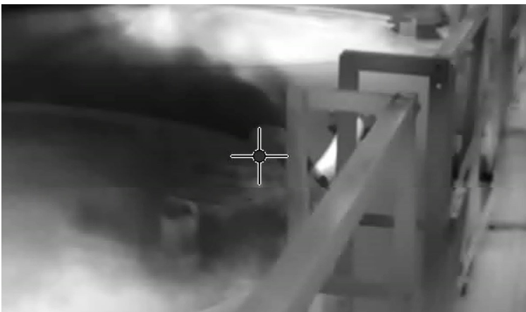
Infrared video image showing emissions from a thief hatch on a storage vessel.
