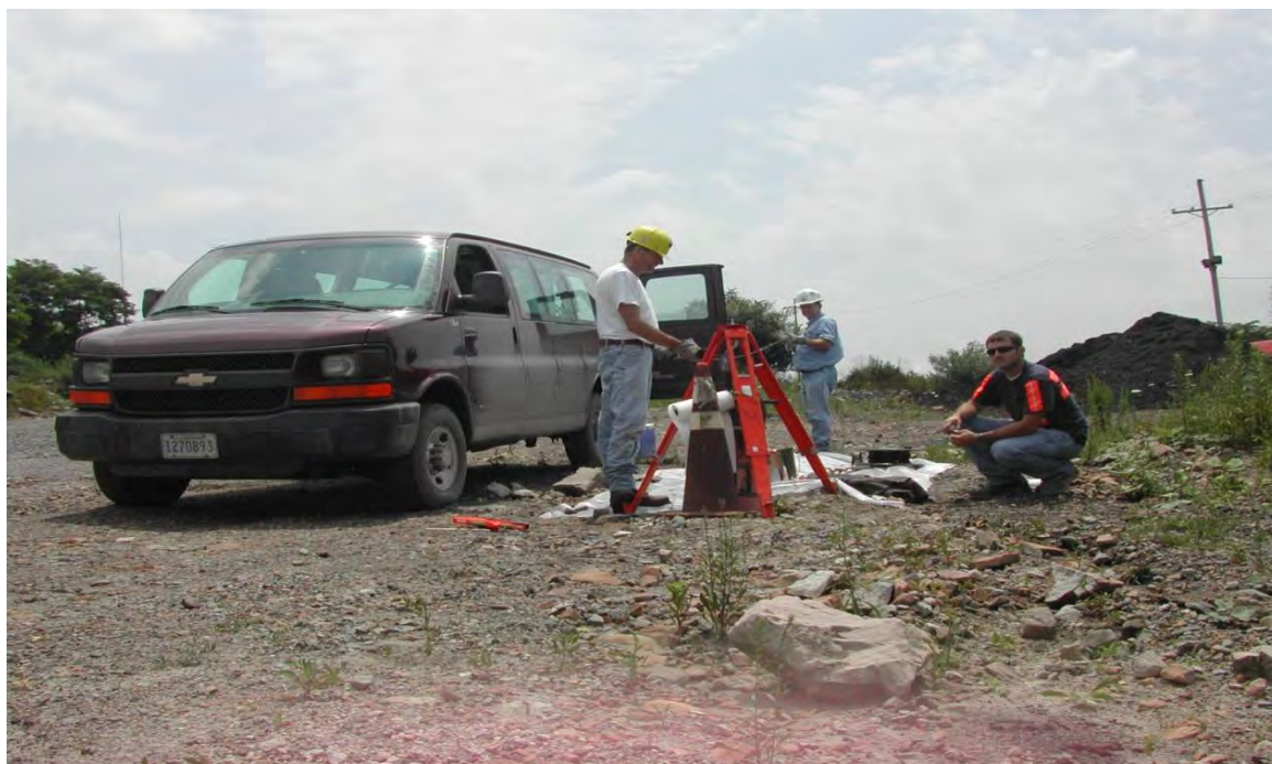
Sampling of monitoring well PM-6 on July 8, 2008. Well is installed in the upgradient portion of the Flying Eagle deep mine.
