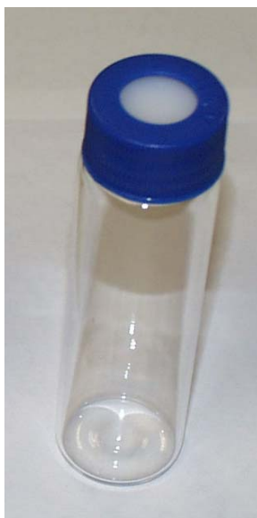
Example of typical vial for VOC and GRO sample collection.
