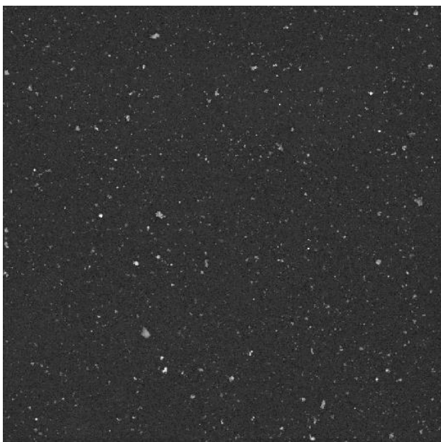
Figure 3 – Medium magnification field from Fig. 1 to analyze particles between 7.5 \mu\text{m} and 2.5 \mu\text{m} . (Field width = 400 \mu\text{m} .)
