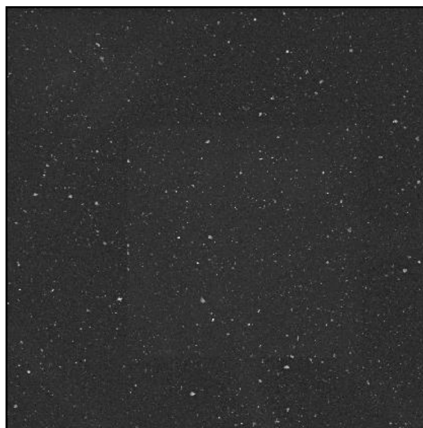
Figure 2 – Low magnification field from Fig. 1 to analyze particles larger than 7.5 \mu\text{m} . (Field width = 800 \mu\text{m} )
