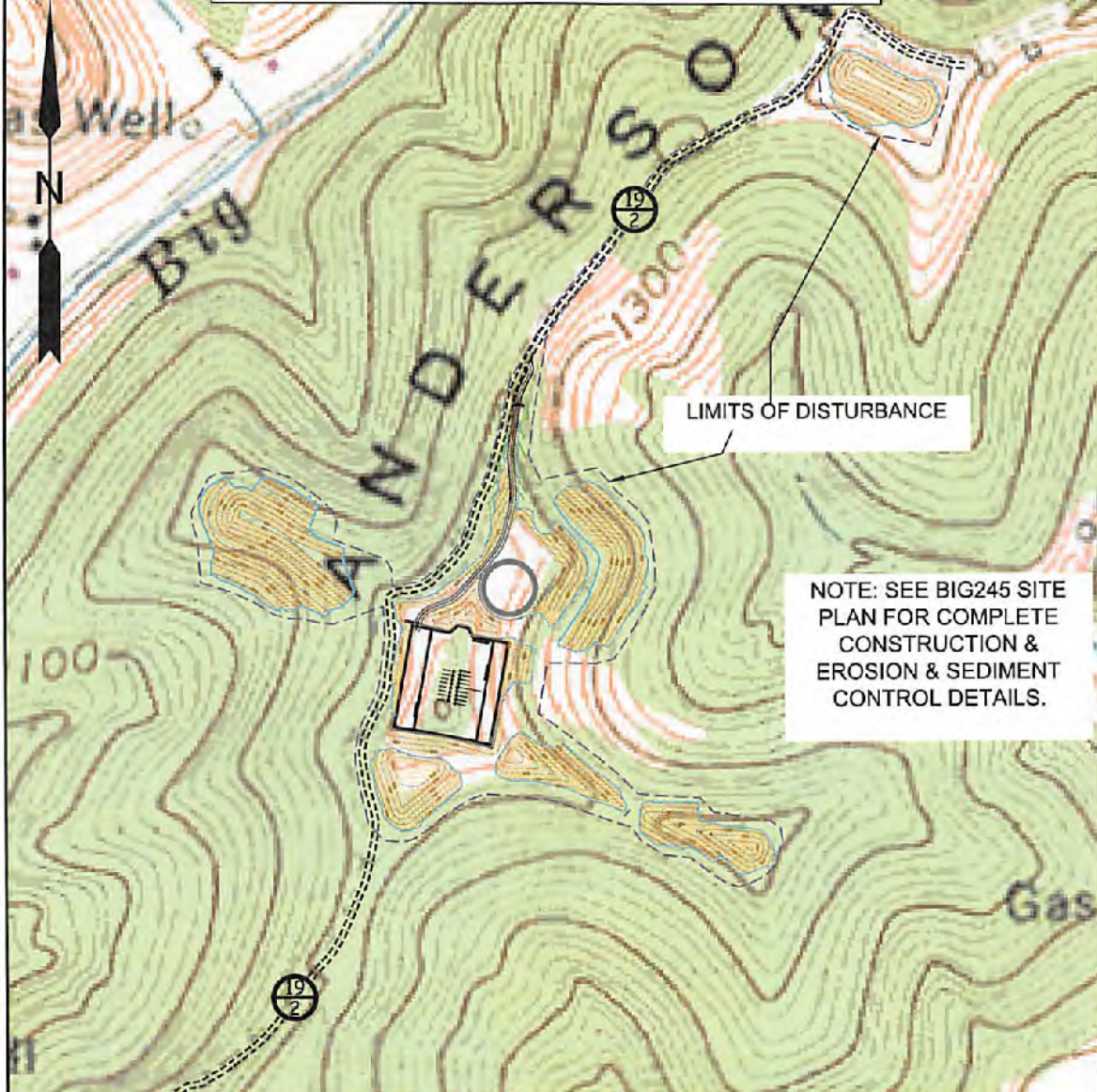
Detail Sketch for Proposed BIG245 Wells
