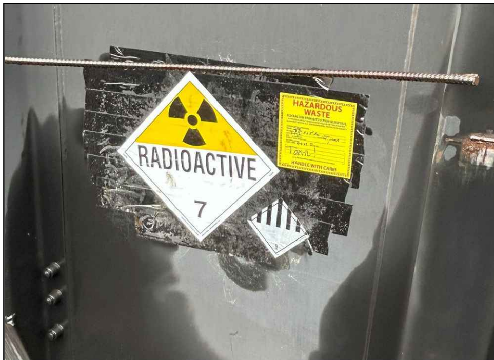
Photo #8 – December 10, 2024: Label added on loaded railcar with “Hazardous Waste”, “Toxic” and accumulation start date. Photo provided by Mr. Isabell, SWVA, Inc.
