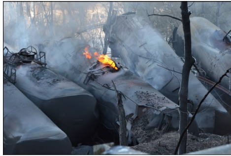
This photograph from Governor Tomblin's Office shows one of the 27 derailed cars burning. The Federal Railroad Administration issued a report Oct. 9 that said the derailment was caused by a broken rail that was missed during inspections.
